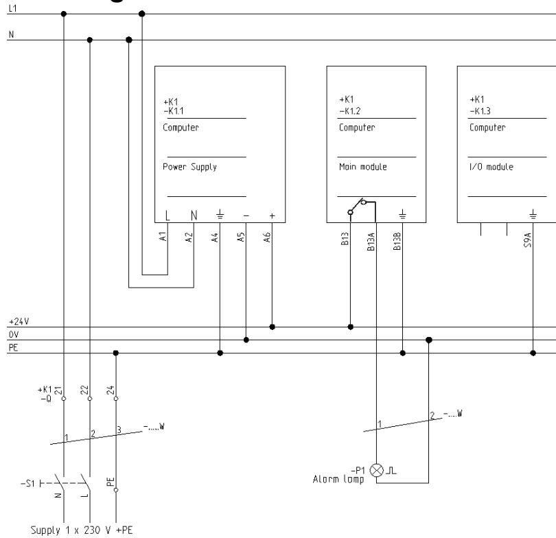
Installation in accordance with applicable national rules; supply cable, however, min. 1.5 mm<sup>2</sup>.
