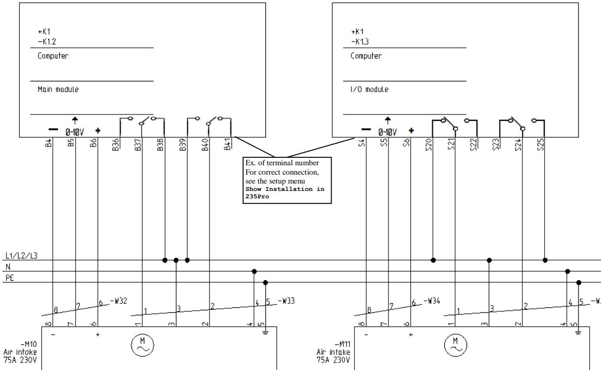
Installation in accordance with applicable national rules. However, cable dimension min. 1.5 mm<sup>2</sup>.
