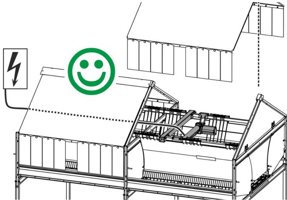
Fig. 2: Drive for expel system installed in nest section, cable guiding correct
