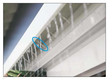
Top profile with perforated pipe and deflector for an even distribution of water along the pads
