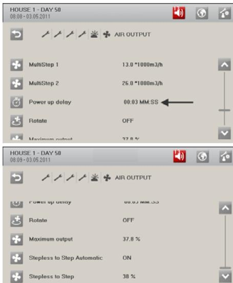
Setting **Power up delay** delays the fan start when restarting after a power failure.
