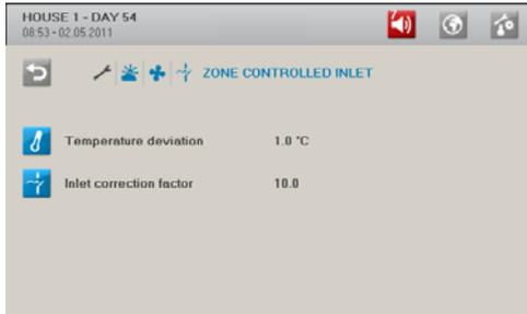
When the zone temperature deviates from **Temperature setpoint** (+ or -), CT2 Touch adjusts the shutter position.
