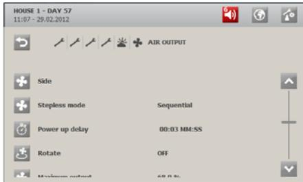
When two stepless fans are used, they can be set up to work in parallel or sequentially.
