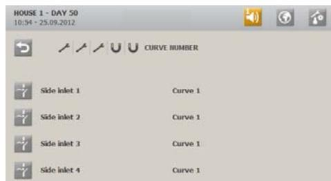
When using more curves, each of max. six air intakes must be associated to the curve according to which it shall be operating.
