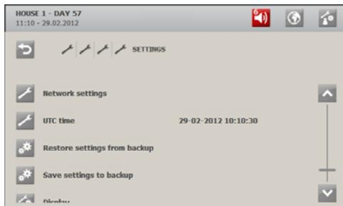
When CT2 Touch's internal SD card is used, it is possible to save and load a backup copy of the current settings.
