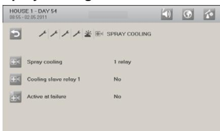
**Yes:** When the control fails, spray cooling is active and runs until the emergency situation is over.
