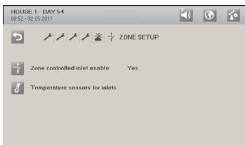
Activate the function in the menu **Technical / Setup / Adjustment / Climate / Zone setup**.
