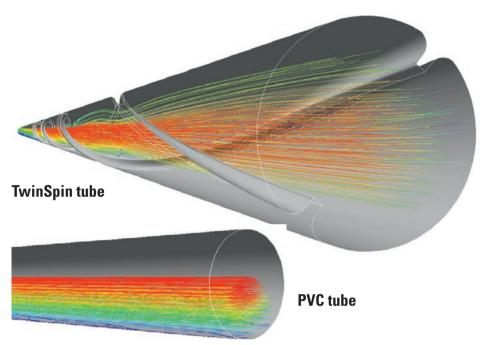
Illustration of the flow velocities in a TwinSpin tube compared with a common PVC tube
